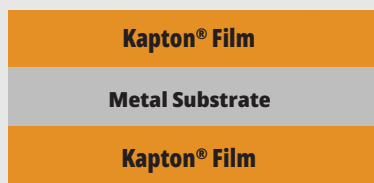
ALT Dura™ (Fralock's Adhesiveless Lamination Technology (ALT™))
